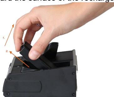
Figure 13: Removing replacement rechargeable battery in the docking station
