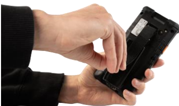
Fig. 51: Closing the Velcro closure of the retaining strap
