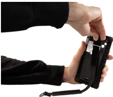
Figure 7: Pulling the retaining strap through the retaining strap attachment
