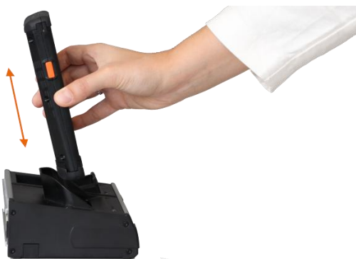
Fig. 53: Inserting Mobile Handheld Computer in and removing it from the docking station
