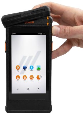
Figure 37: Removing the upper logistics protective cap
