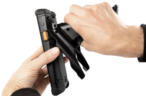
Figure 31: Attaching M2Grip5/M2Grip5 SE to M2Smart®SE
