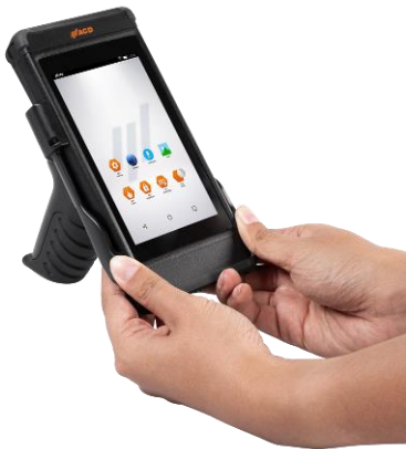
Fig. 74: Removing M2Grip5/M2Grip5 SE from M2Smart®SE (1/2)
