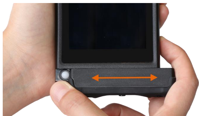
Figure 25: Attaching and removing the lower plug-in module
