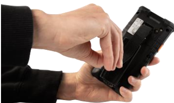
Figure 9: Closing the Velcro closure of the retaining strap
