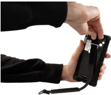
Fig. 49: Pulling the retaining strap through the retaining strap attachment
