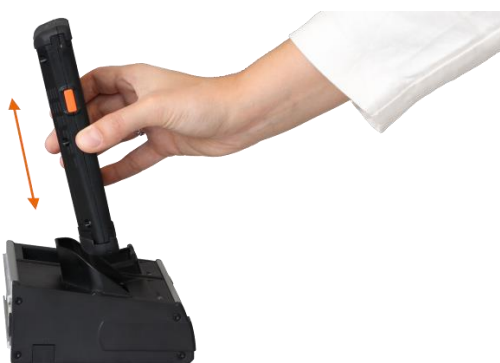
Figure 11: Inserting Mobile Handheld Computer in and removing it from the docking station
