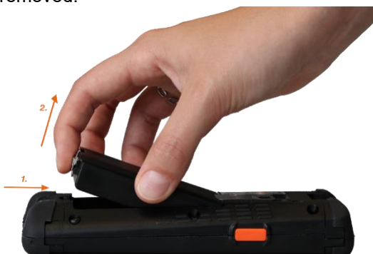
Figure 1: Removing the rechargeable battery
