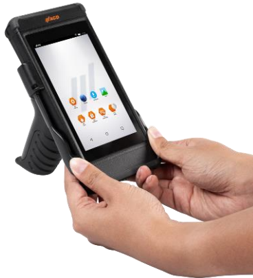
Figure 32: Removing M2Grip5/M2Grip5 SE from M2Smart®SE (1/2)
