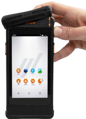
Figure 35: Attaching the upper logistics protective cap
