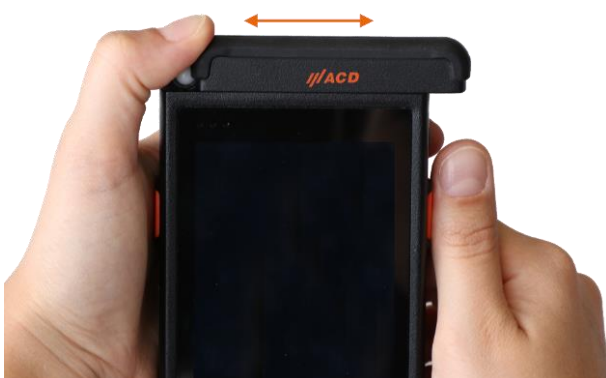
Figure 24: Attaching and removing the upper plug-in module
