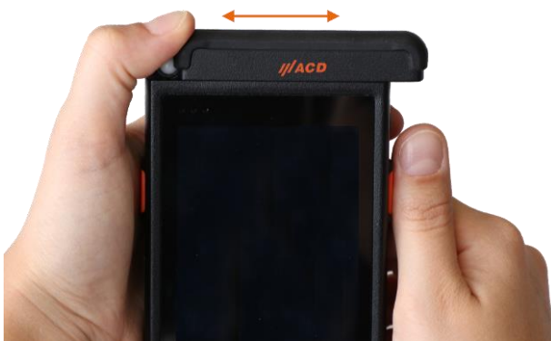
Fig. 66: Attaching and removing the upper plug-in module
