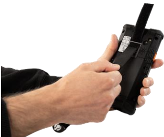
Fig. 48: Pulling out the retaining strap down
