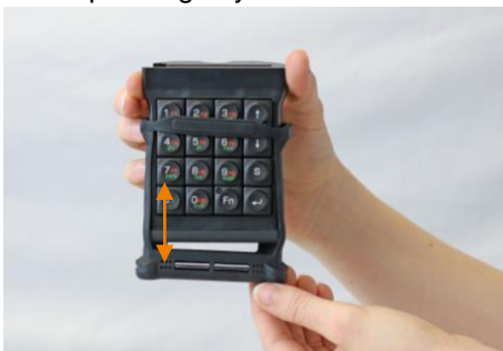
Fig. 82: Attaching the M2Key16 Logistics protective cap
