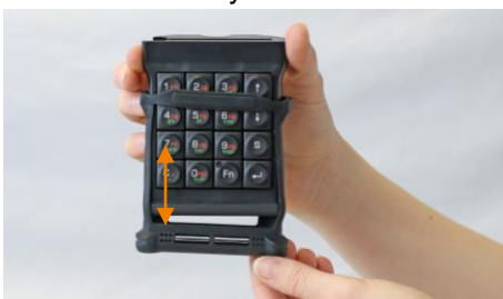
Figure 41: Removing the M2Key16 Logistics protective cap
