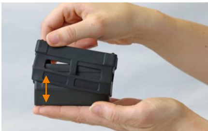
Fig. 85: Attaching the M2Longrange protective cap
