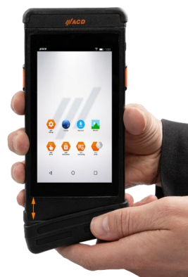
Figure 38: Removing the lower logistics protective cap
