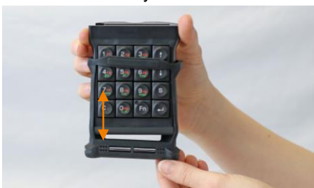
Fig. 83: Removing the M2Key16 Logistics protective cap
