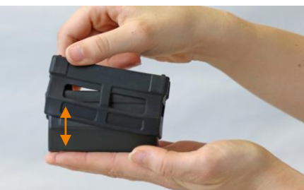
Fig. 86: Removing the M2Longrange protective cap
