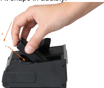
Figure 12: Inserting replacement rechargeable battery in the docking station
