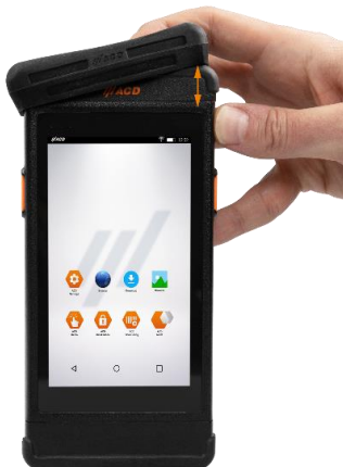
Fig. 79: Removing the upper logistics protective cap
