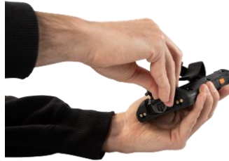
Fig. 47: Detaching the retaining strap eyelet
