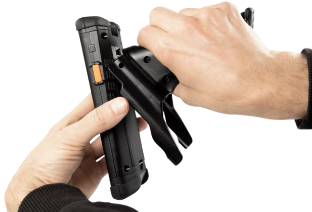
Fig. 75: Removing M2Grip5/ M2Grip5 SE from M2Smart®SE (2/2)
