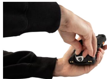
Fig. 50: Attaching the retaining strap eyelet
