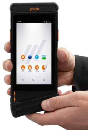
Fig. 80: Removing the lower logistics protective cap
