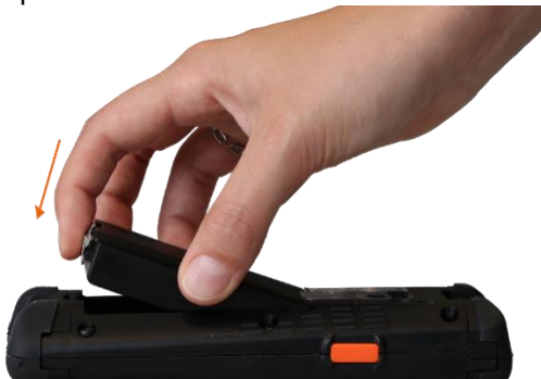
Fig. 45: Inserting the rechargeable battery
