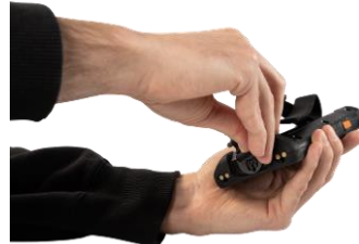
Figure 5: Detaching the retaining strap eyelet
