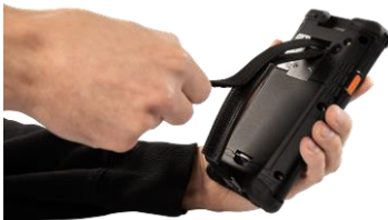
Figure 4: Opening the Velcro closure of the retaining strap
