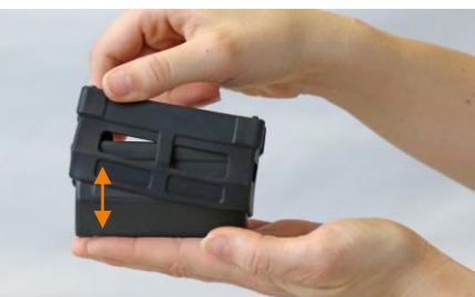
Figure 44: Removing the M2Longrange protective cap
