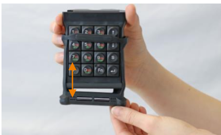
Figure 40: Attaching the M2Key16 Logistics protective cap
