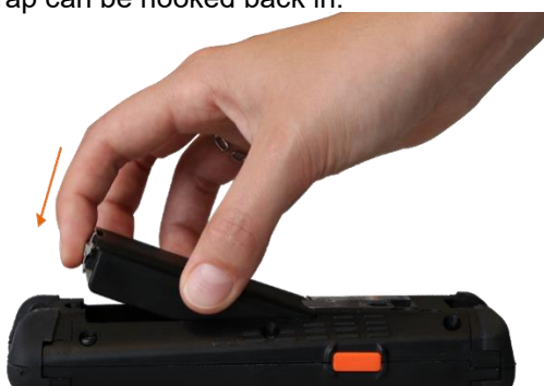
Figure 2: Inserting the rechargeable battery
