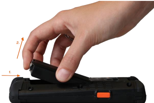
Fig. 44: Removing the rechargeable battery
