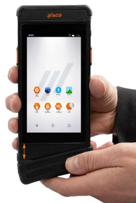
Figure 36: Attaching the lower logistics protective cap
