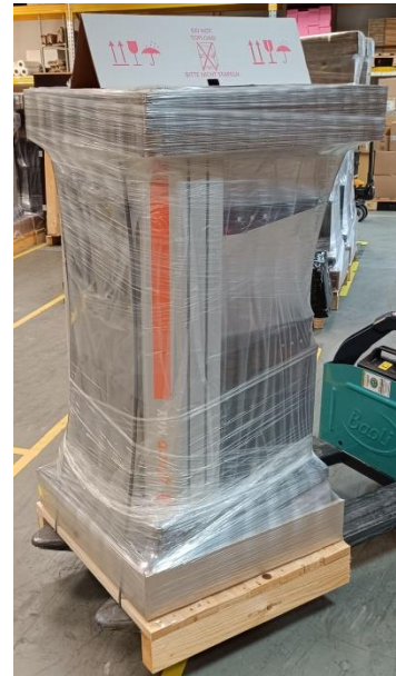
Figure 8: Wrapping the MAX BE with foil
