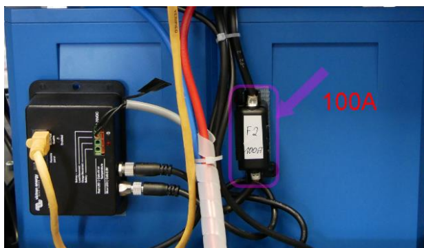
Figure 34: MAX BE 750/1200 Li-Ion and MAX Plus 750/1200 Li-Ion fuses on the battery
