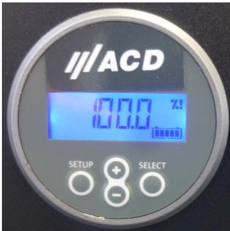
Figure 25: Battery controller MAX BE Li-Ion and MAX Plus Li-Ion
