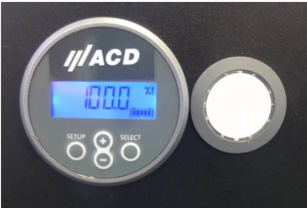
Figure 23: Battery controller, On/Off switch
