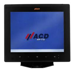
In addition to the well-established MFT1xSE variants with 10.4" and 12.1" displays, our Second Edition is now also available with a 15" display. The MFT15SE completes the product portfolio of forklift terminals and ACD Elektronik can now provide the suitable forklift terminal for every application in the logistics and warehouse environment.
