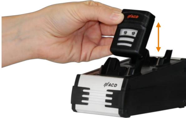
Figure 3: Inserting the wearable scanner in and removing it from the docking station
