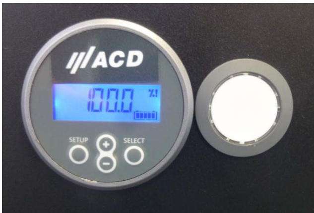
Figure 23: Battery controller, On/Off switch
