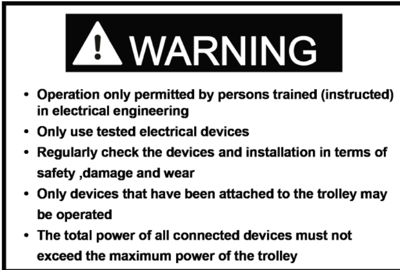
Figure 3: Warning sign under the table top of the mobile workstation
