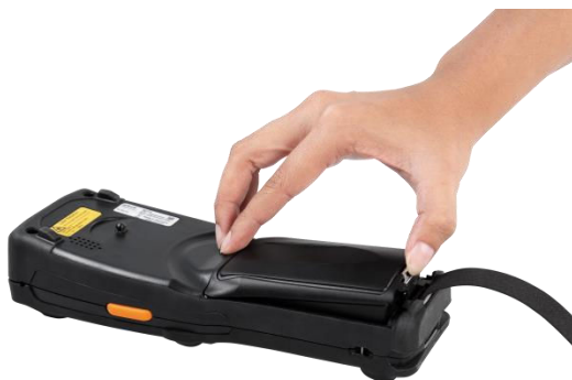
Fig. 8: Changing the battery
