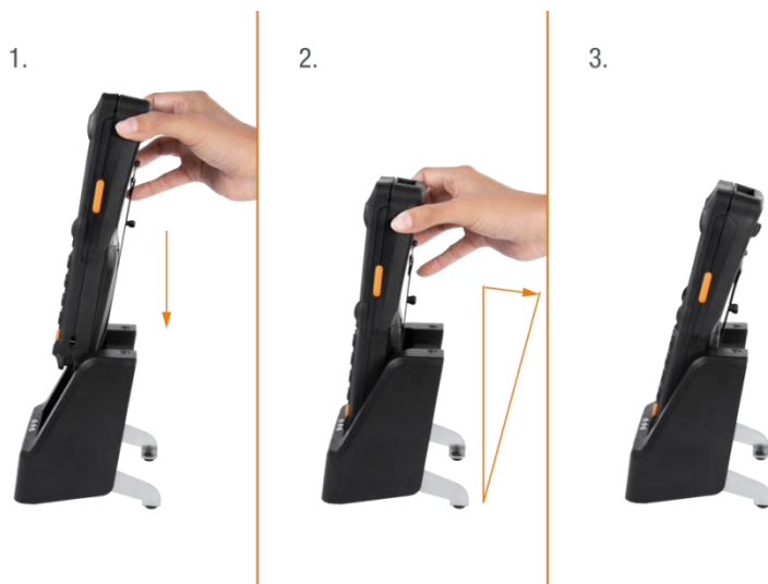
Fig. 9: Inserting the Mobile Handheld Computer into the docking station
