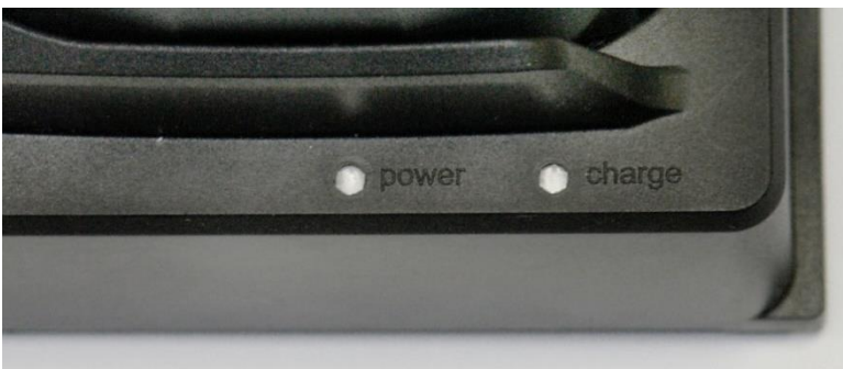
Fig.14: Spare Battery Charger Status LEDs
