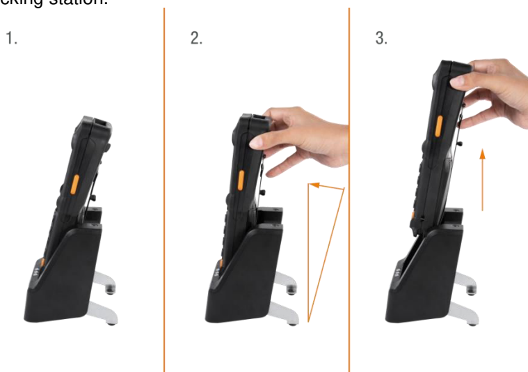
Fig. 10: Removing the Mobile Handheld Computer from the docking station
