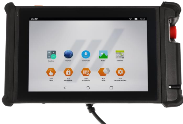
Figure 3: Front view with the emergency stop button
