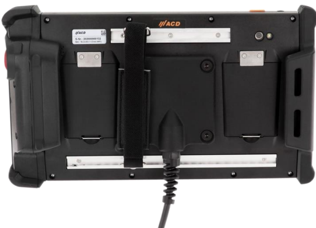
Figure 5: Rear view without enabling switch
