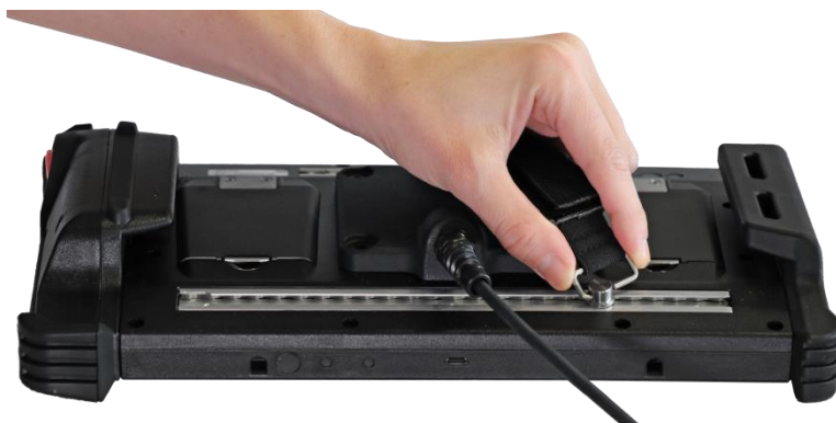
Figure 16: Retaining strap loosening/adjusting
